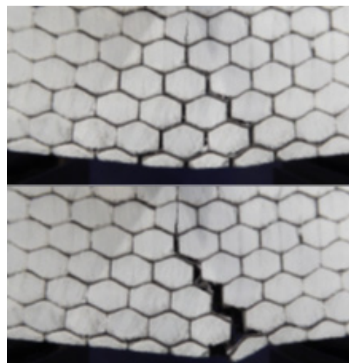
Figures: Schematic drawing of a force/displacement curve in a three-point bending test of a monolithic ceramic (brittle failure) vs. a digital ceramic (ductile stepwise failure) on the top and such an example on the bottom prior to complete failure.
