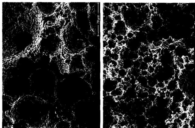
Fig. 3: Effect of the emulsifier concentration on the microstructure of CPC – oil mixtures after washing off the oil and sintering. After sintering, the blocks consisted of  $\beta$ -TCP.
