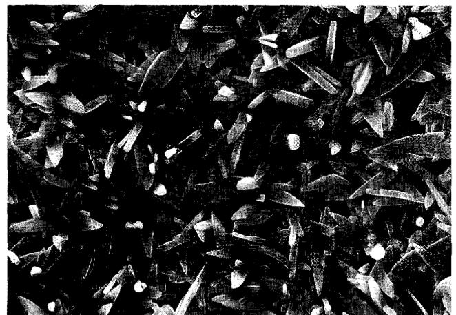
Fig. 2: Typical microstructure of a brushite CPC. Crystal entanglement providing mechanical rigidity to the cement. Micropores are formed by the intercrystalline space.
