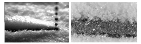
**Fig. 4.** High speed frame (left) of the droplet impact on the powder bed. Detail of a line (right) lying in the wide groove formed within the bed. (Reprinted from *Rapid Prototyping Journal*, 2003, © Emerald Group Publishing Limited, all rights reserved.)
