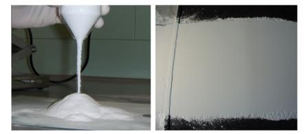
Fig. 8. High flowability of plasma treated 5 µm powder (left) and a homogeneous bed of the same powder (right).
