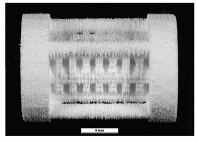
Fig. 6. 3D printed calcium phosphate scaffold.
