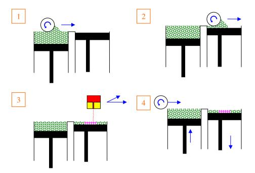
**Fig. 2.** Iterative steps in the powder-based 3DP principle. The roller places a thin layer of powder in the build area (steps 1 and 2). The inkjet head prints droplets of a binder fluid on the powder bed and thus locally solidifies part of the solid cross-section (step 3). This process is repeated for every layer until the 3D structure is printed and the remaining powder is removed (step 4).
