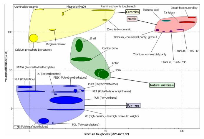
Fig. 1. Mechanical properties of natural materials in comparison with bulk materials for medical purpose (graph constructed with CES Selector 5.1.0).
