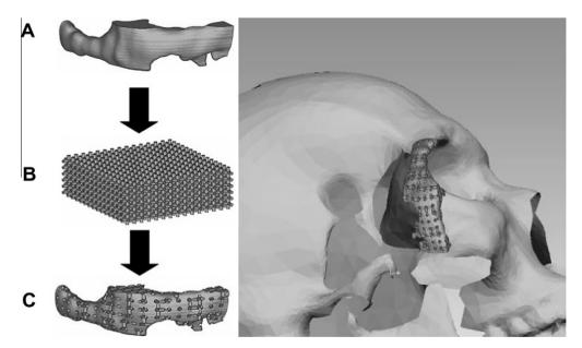
Fig. 7. Virtual construction steps of 3D printed skull scaffold. (Reprinted from Materialwissenschaft und Werkstofftechnik, © 2006, permission from Wiley being sought.)
