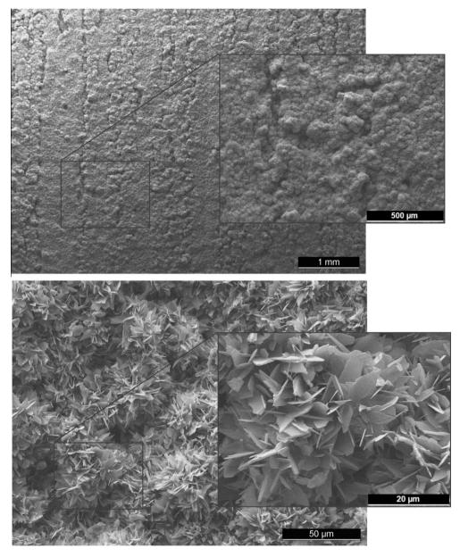
Fig. 5. 3DP surface structure after the reaction between TCP and the acid binder. Four enlargements of a 3D printed surface are shown.
