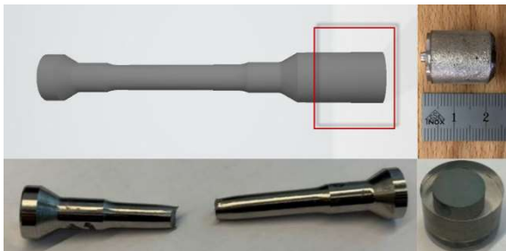
Fig. 1: Tensile tests sample with integrated microsection specimen (red box).
