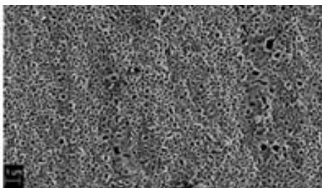
Fig. 1 SEM micrograph of dark green anodized sample with a 5% duty cycle (on-off time) in 2.8 M H 2 SO 4 . (1 micron marker in lower left).
