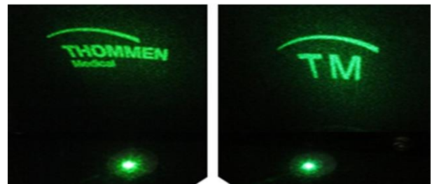
Fig. 2: A DOE-diffracted laser produces a visible, precalculated image on a screen.
