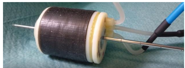
Fig. 2: 3D printed multimaterial pneumatic medical biopsy actuator after gamma irradiation.
