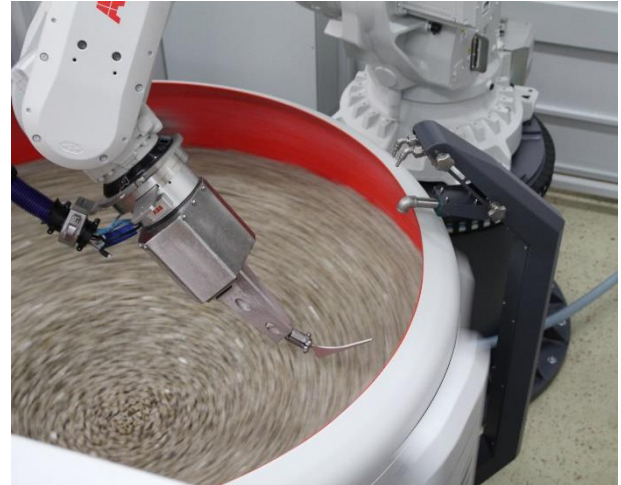
Fig. 2: The robot fulfils not only a material handling function but also guides the work pieces through the processing medium during the finishing cycle.
