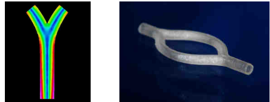
Fig. 1: Left: Computational evaluation of wall shear stress. Right: prototype of a branched tube, fabricated from newly developed cytocompatible elastomeric material by UV laser curing.
