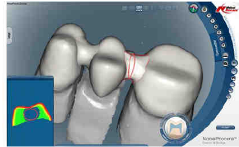
Fig. 2: CAD design of a zirconia bridge in the NobelProcera™ Software.
