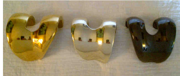
Fig. 1: left: PVD-Medthin™ 01 TiN. TiN is FDA approved since 2002 and sold in USA, Europe, Australia and emergent markets, etc; middle: PVD multilayer Ionbond-Aesculap AS coating 510K approved, on sale in USA, Europe and other countries; right: CVD dual and multilayers coatings by Ionbond.
