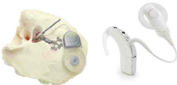
Fig. 1: Implantable hearing aid DACS (direct acoustic cochlear stimulation) with external sound processor.
