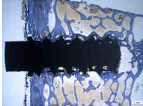
Fig.1: Histology at 8 w – Ti A.M. Macroporous Surface. Bone ingrowth visible inside pores
