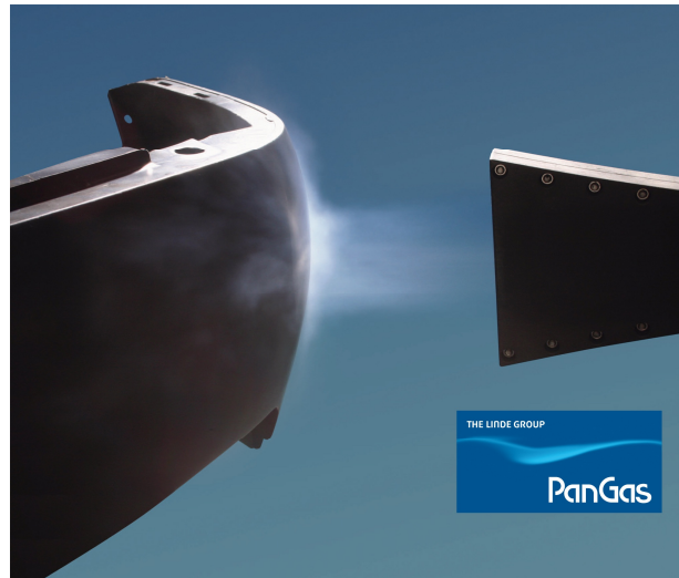
Fig. 1: CRYOCLEAN® snow pretreatment of a plastic part prior to a painting process.
