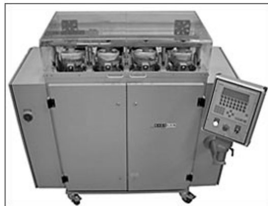
Fig. 1: EndoLab ® ISO 14243-1 knee simulator.
